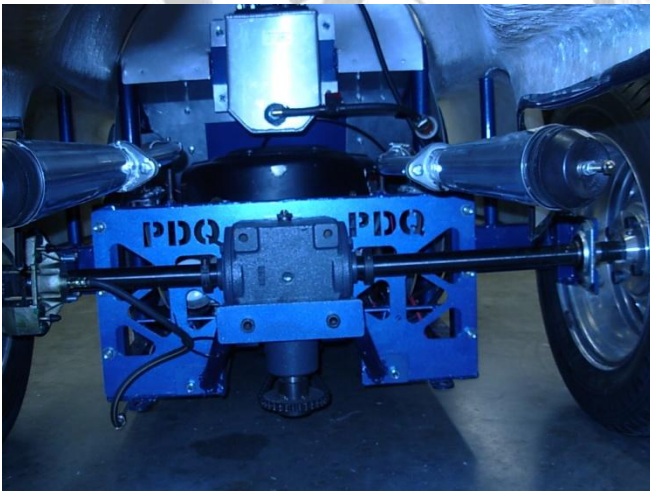
The back of the car with the exhaust, fuel tank, and rear axle installed
